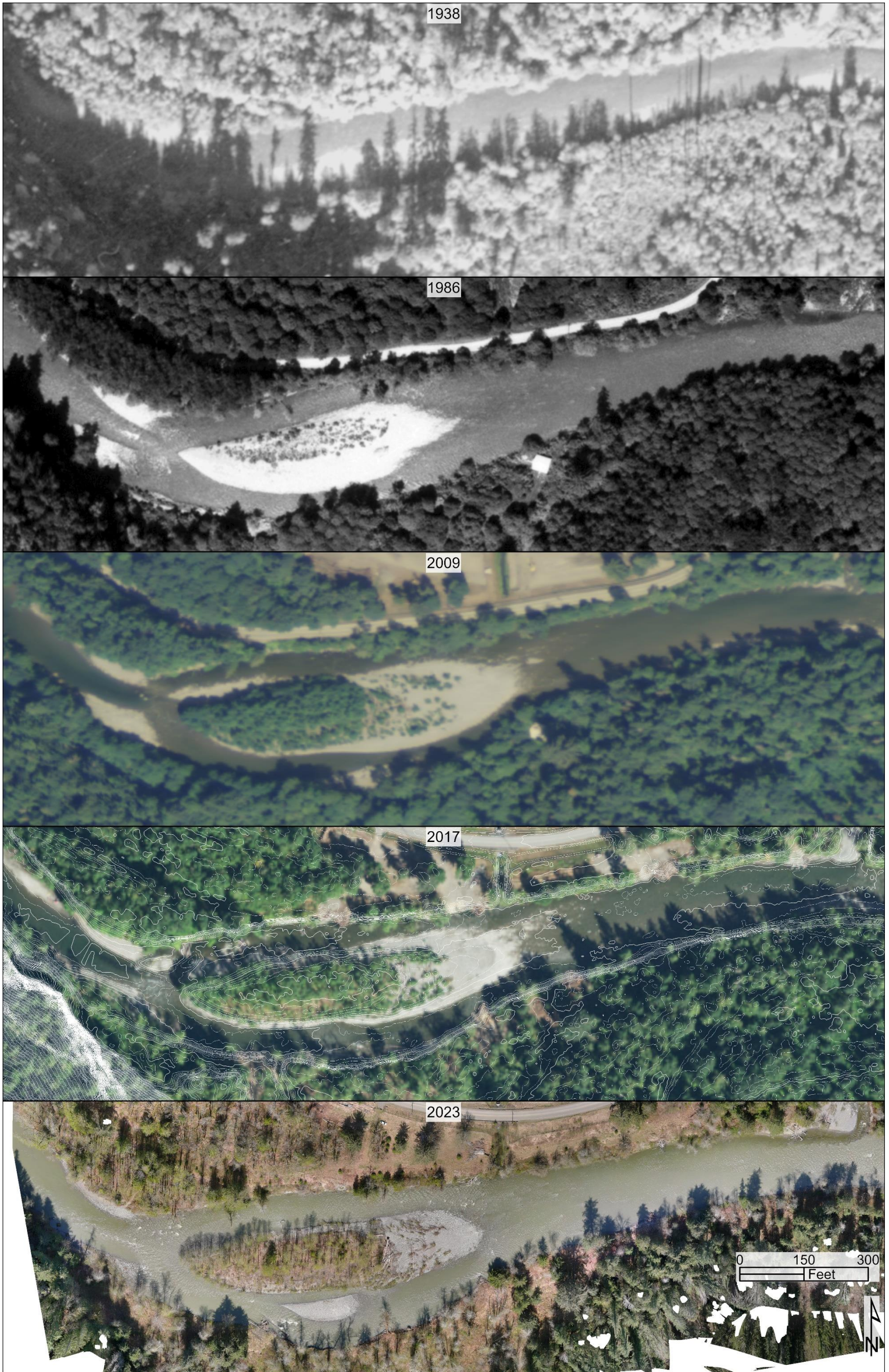
Figure 2: Historical geomorphic evolution of the project reach from 1938 to 2023. 2017 imagery has 1-ft topobathymetric contours.
