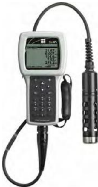
Figure 2.1 Photo of YSI 556 Showing Hand-Held Instrument, Cable, and Sonde Fitted with Probe Guard
